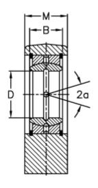
$\begin{array}{lll} A & = 100 \\ a \text{ (degrees)} & = 7 \\ B & = 28 \\ D & = 40 \\ Dynamic load C \text{ (kN)} = 100 \\ F & = 69 \\ L & = 119 \\ \end{array}$
